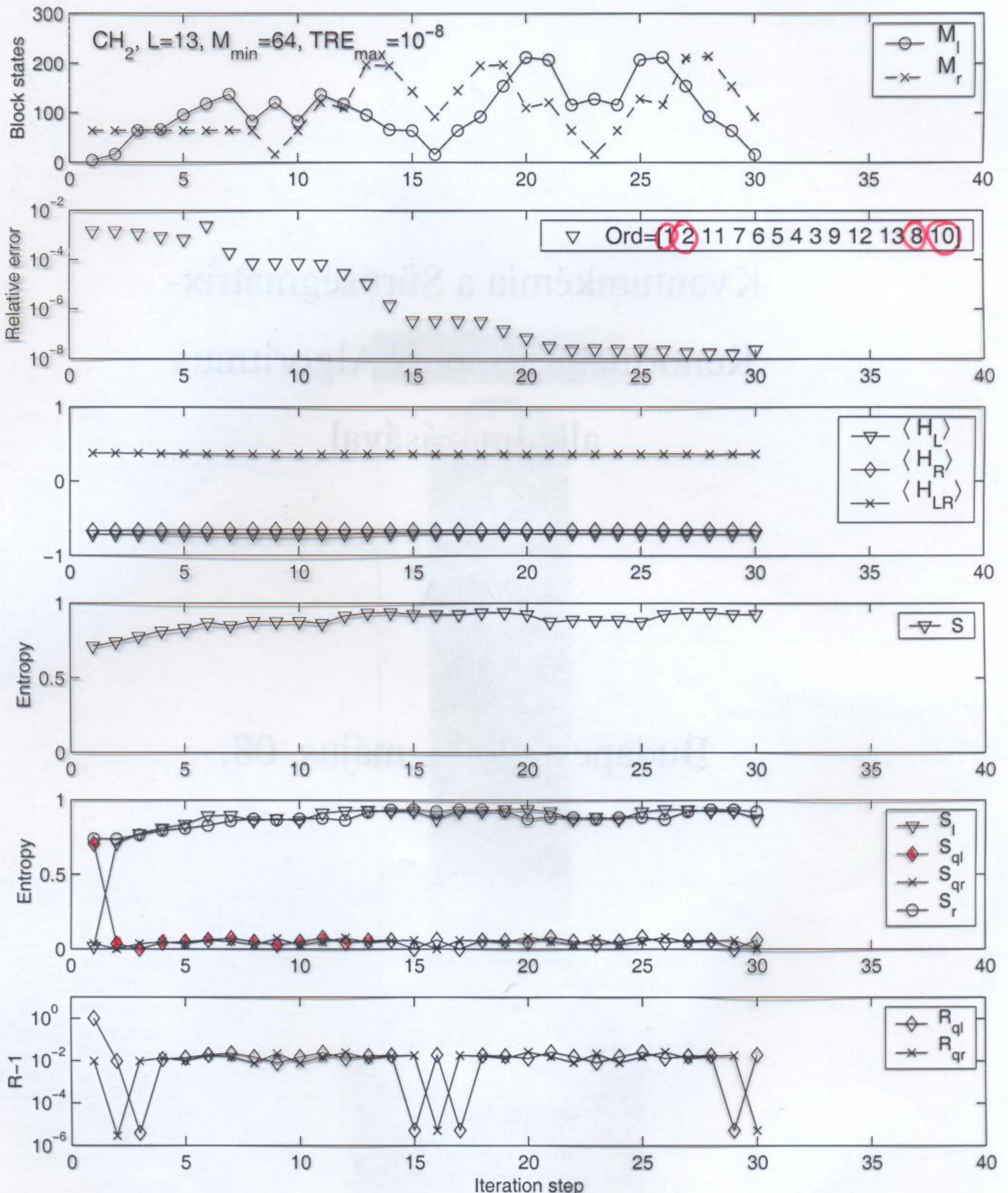
FIG. 5. Same as Fig. 4 but for an ordering when relevant information of the system is shared between DMRG system blocks giving rise to strong interblock interaction and large quantum information exchange between the blocks.
