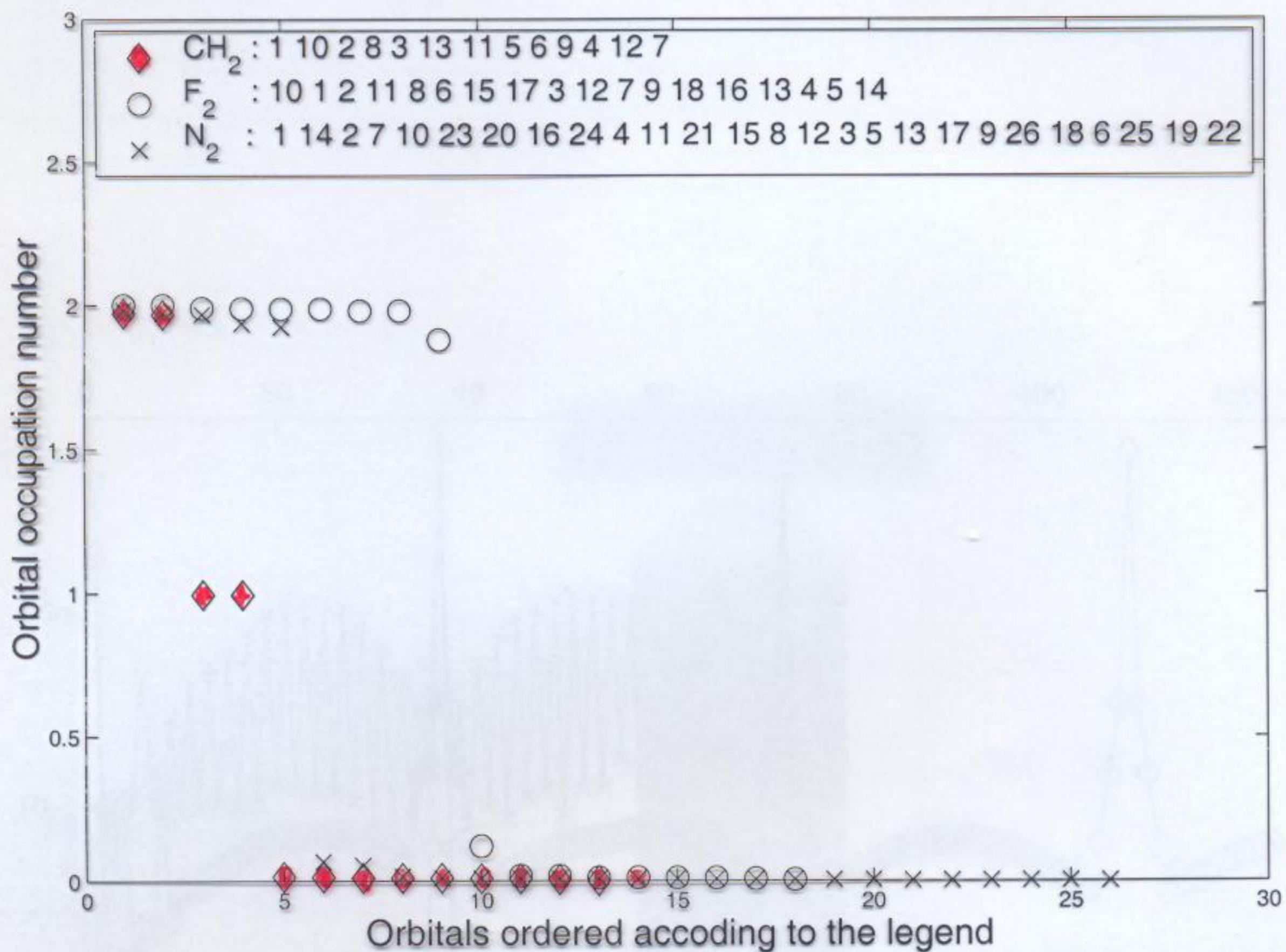
FIG. 3. Decay of orbital occupation number obtained in the full CI limit and the corresponding ordering of orbitals for molecules studied in the paper.
